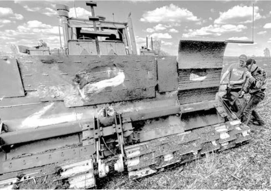
Farmers fix remote-controlled demining machine near Kharkiv, Ukraine, April 26. Oleksandr Kryvtsov protects his tractor from explosions with armor plates from destroyed Russian tanks.
